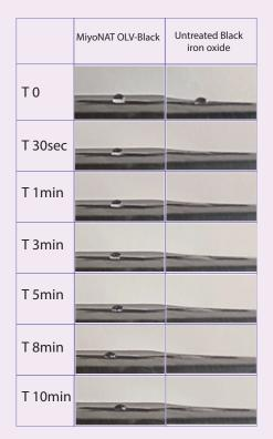
**Conclusion :** MiyoNAT OLV treatment displays a really high hydrophobicity.
